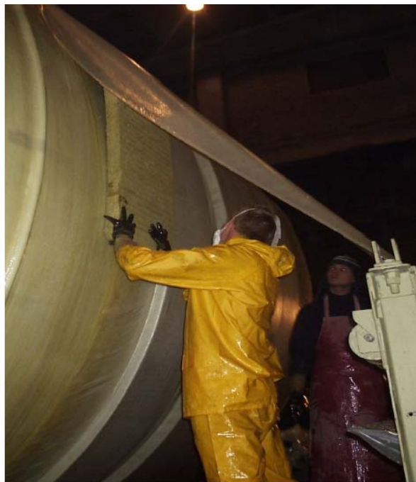
Production of «Sandwich» FRP shell
