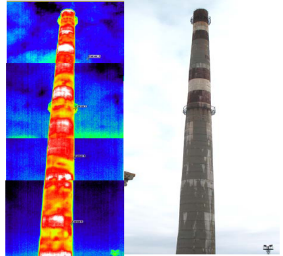
Typical state of RC chimney (inspection results)
